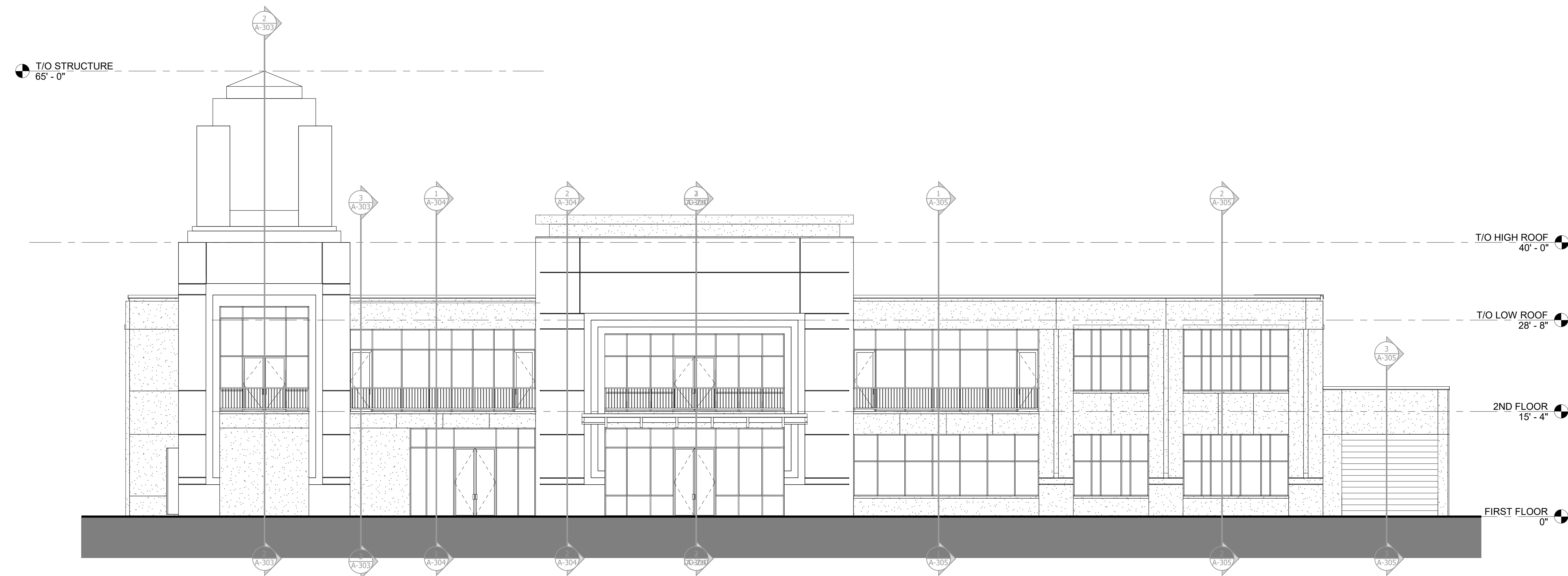
EAST EXTERIOR ELEVATION 1/8" = 1'-0"
